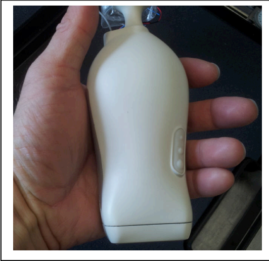
Figure 1: Prototype of the handheld FULLPHASE PA probe.
